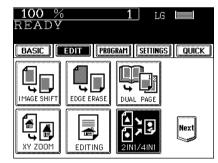
Select the type of image combination. - Press the 2IN1 (or (4IN1), (2IN1), (DUPLEX) or (4IN1 DUPLEX)) key.
